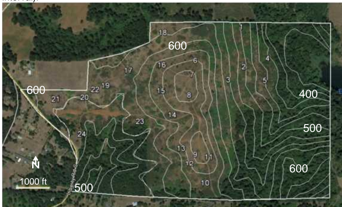
Figure 3. Topographic map of the property with soil boring locations (25 ft. contour interval).
